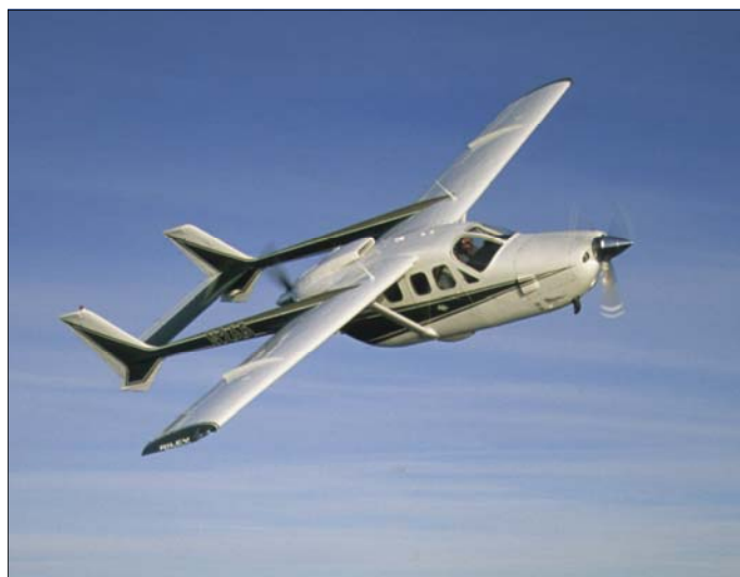
The Cessna 337 Skymaster is a fast, beautiful airplane with twin engines, one pusher and one puller.
