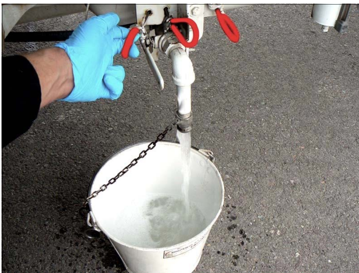
Performing a visual appearance test using a white bucket to detect the presence of water or solid contamination. Photo by Chris Hart.
