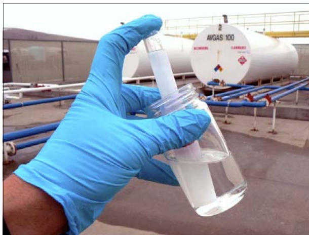
The Hydrokit test detects the presence of suspended water in jet fuel. Photo by Chris Hart.
