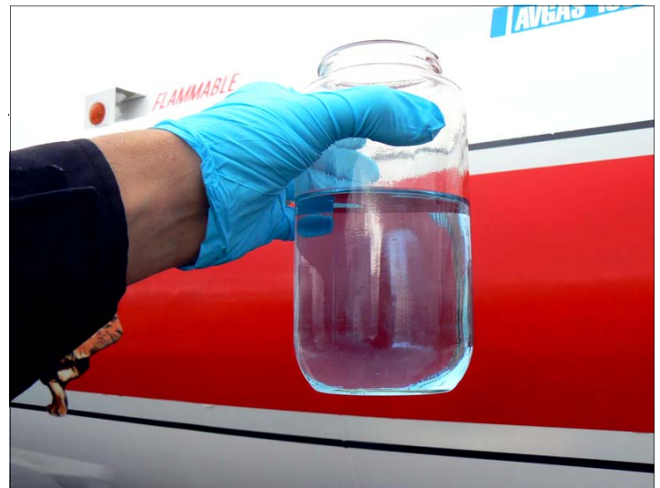
The clear and bright test is performed to verify the proper grade of fuel and to detect water or solid particulates. Photo by Chris Hart
