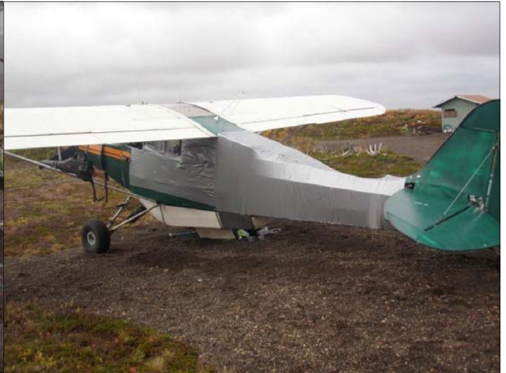
With 2 new wheels and lots of duct tape, the plane was flown out of the back country airstrip.
